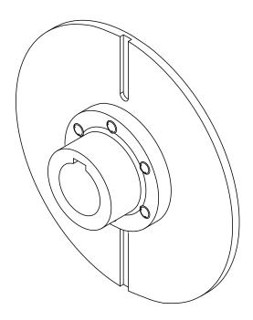
**Note:** This armature assembly is balanced and care must be taken to keep it flat and true. Caution should be used when following instructions shown below.
